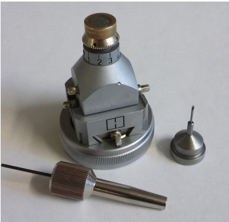
Figure 5, Goniometer head with magnetic snap on mount and adjustment screw
